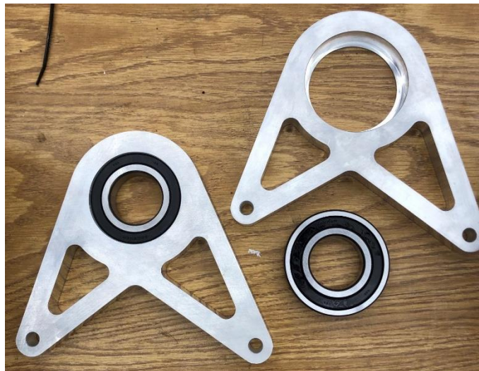
Figure 21: Differential frame fabricated
